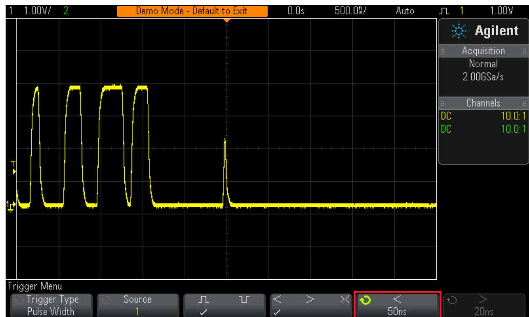
Figure 27 Triggering on a narrow infrequent glitch using the scope's Pulse Width triggering mode.
